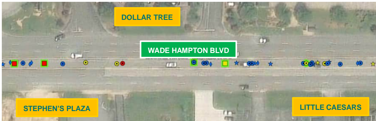
Section of US 29 just south of Tappan Drive. Pedestrian (red icon, outlined in green) and vehicle fatal crashes (red icon, no outline) and angles occurred in this section.
